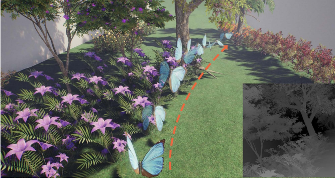
Fig. 10. The simulated insect flies freely in a virtual natural environment, avoiding obstacles through visual perception. The lower-right presents the corresponding visual depth image.
